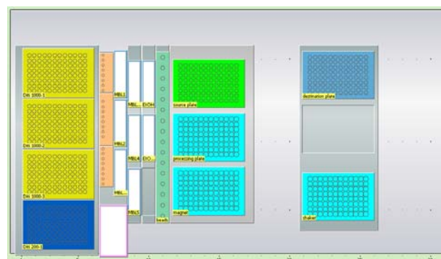
Figure 1 Worktable layout for high throughput isolation of DNA from whole blood using Tecan's Te-Shake and MACHEREY-NAGEL's magnetic separator.
