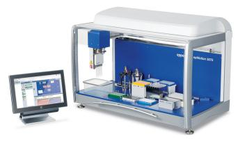
This protocol is programmed to process up to 24 samples in parallel and developed for the ep*Motion*® 5075vt platform.
