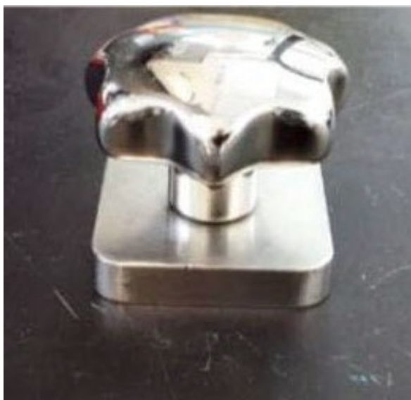
Figure 11. Blot the chip with Blotting Paper and Blotter. A Blotter is provided with the ICELL8 Single-Cell System.
