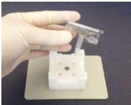
Figure 49. Removing the Collection Tube containing the eluate.
