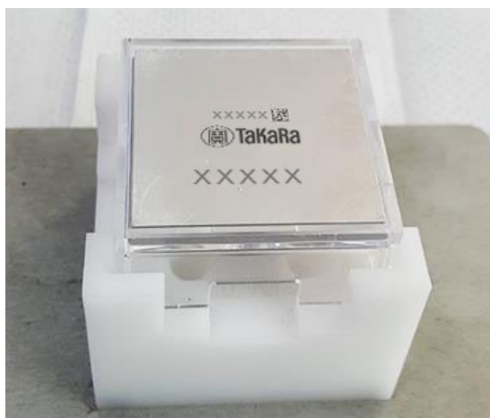
Figure 47. Placing the chip into the collection module.
