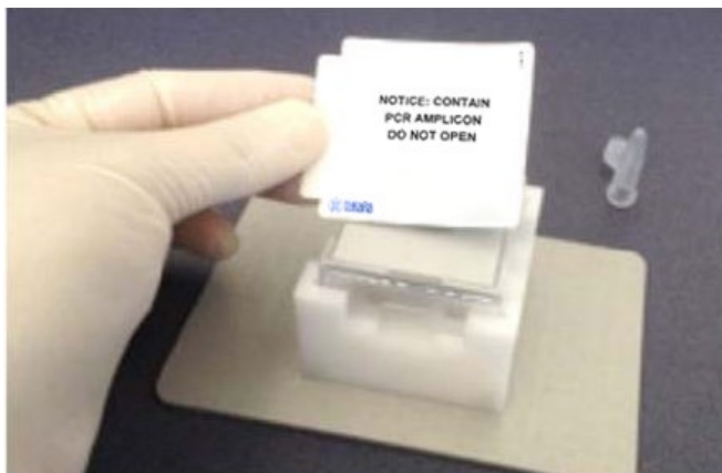
Figure 48. Securing the collection module with Collection Film.
