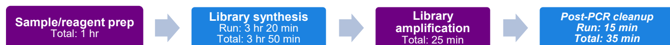
Figure 1. Library preparation workflow overview for one batch of up to 32 samples on the Apollo system with the PrepX ILMN DNA Library Kit - B. Blue and purple boxes indicate steps performed on and off the Apollo system, respectively. The italicized text indicates that the post-PCR cleanup requires a separate protocol. Run = the run time in minutes on the Apollo system, if applicable. Total = total time in minutes spent, including thawing of reagents, reagent and equipment setup, heating and cooling of thermal blocks, incubation of reactions, and automated liquid-handling processes, if applicable.
