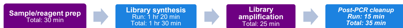
Figure 1. Library preparation workflow overview for one batch of up to eight samples on the SMARTer Apollo system with the SMARTer PrepX DNA Library Kit - A. Blue and purple boxes indicate steps performed on and off the SMARTer Apollo system, respectively. The italicized text indicates that the post-PCR cleanup requires a separate protocol. Run = the run time in minutes on the SMARTer Apollo system, if applicable. Total = total time in minutes spent, including thawing of reagents, reagent and equipment setup, heating and cooling of thermal blocks, incubation of reactions, and automated liquid-handling processes, if applicable.
