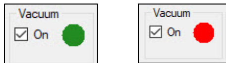
Figure 73. Vacuum status confirmation. (Left) The minimum vacuum level has been reached. (Right) Insufficient vacuum level indicator.
