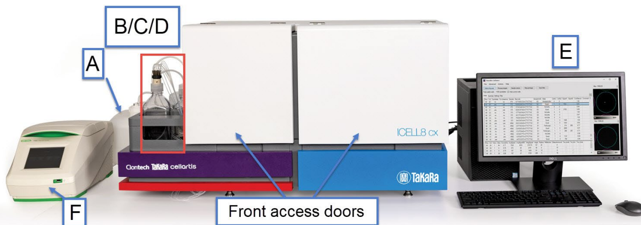
Figure 2. The ICCELL8 cx Instrument (external view). This image is for Cat. No. 640188. Note: A thermal cycler (F) is not included in Cat. No. 640189.
