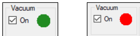
Figure 73. Vacuum status confirmation. (Left) The minimum vacuum level has been reached. (Right) Insufficient vacuum level indicator.
