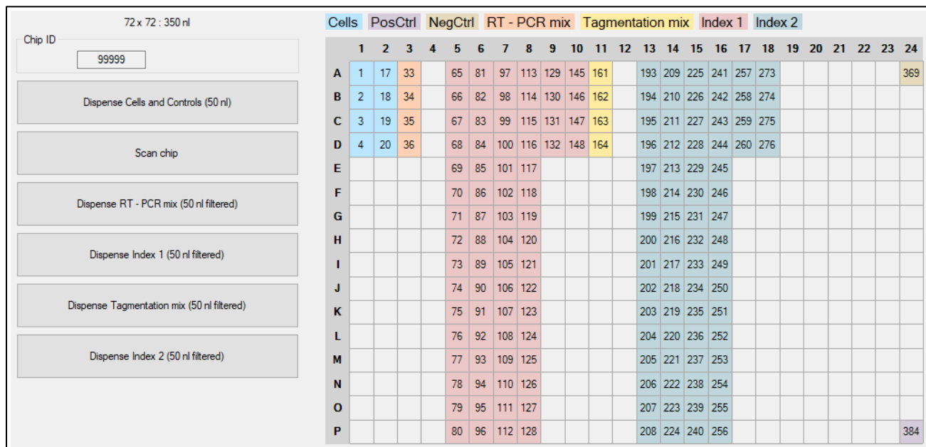
Figure 105. Source well map for dispenses in an example SMART-Seq full-length analysis run.
