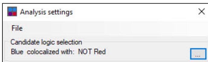
Figure 8. Accessing the Candidate Logic Selection window for the V2 algorithm. The [...] is clicked to bring up the window to configure the logic rules.
