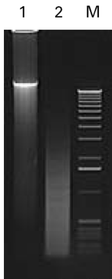
Figure 3. E. coli genomic DNA before (Lane 1) and after (Lane 2) Rsa I digestion. Lane M:DNA size markers.
