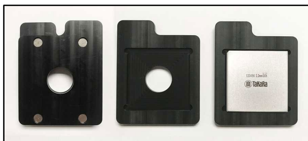
Figure 12. Nanodispenser Chip Holder.
