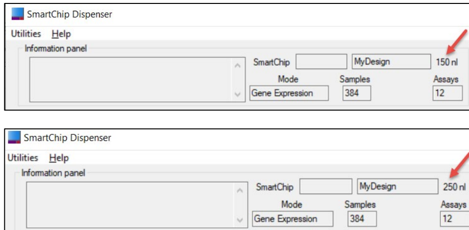
Figure 24. Finding the selected chip well volume. After selecting the size of the chip (Figure 23), the related volume will display on the main UI. Top: 150 nl. Bottom: 250 nl.
