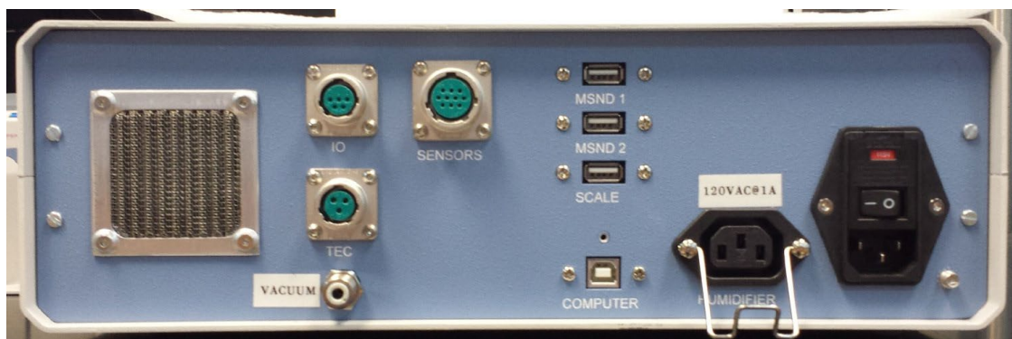
Figure 6. Connections on the rear of the peristaltic pump control box.
