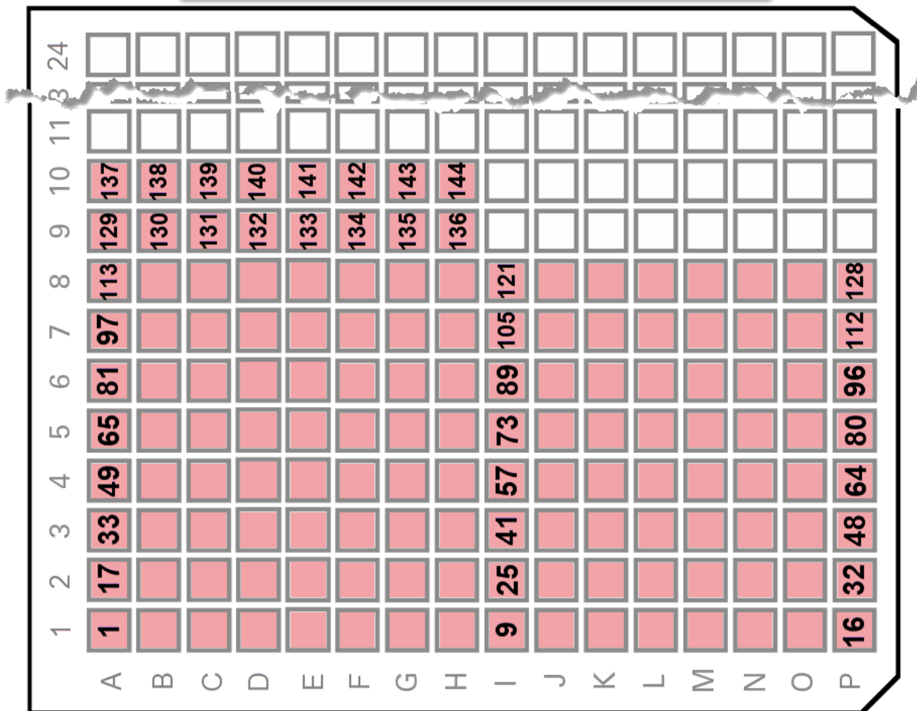
Figure 78. Printable 384-well plate map (partial) for dispense of 144 samples or assays into a MyDesign chip.
